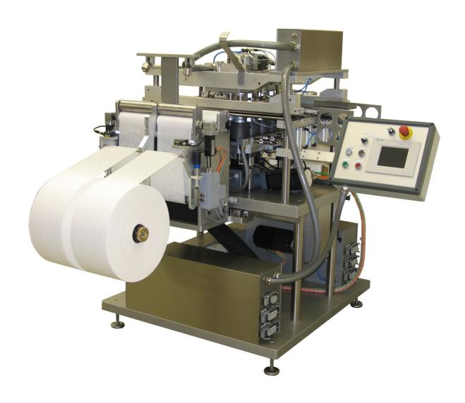
8-fold sealing machine cycle rate 80 per minute
